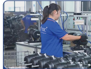
AIR LEAKAGE TESTING
